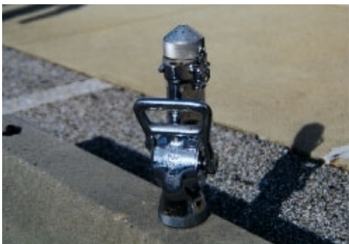
In the early 1950s, Akron Brass introduced a periphery jet fog nozzle known as the "PDQ."
