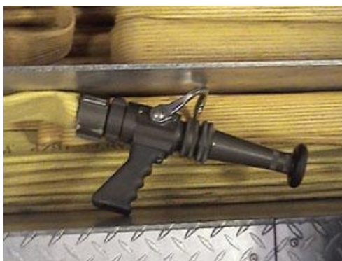
(2) The new 1 \frac{5}{16} -inch smooth bore nozzle, which has a stream shaper.
